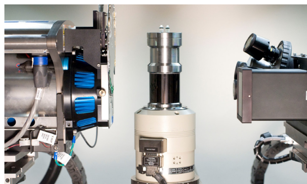
Figure 1 ZEISS Xradia Versa with X-ray source (left), sample stage with tension/compression stage (center), and detector (right). Even with source to sample distances of several centimeters, required to accommodate in situ sample holders, voxel sizes below one micron can be achieved.
